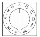
Use this control knob to select the oven function and turn on the oven light in the secondary oven.
