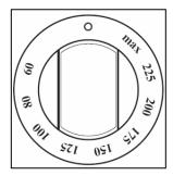
The oven thermostat control knob should be turned clockwise and it sets the required temperature of the oven. It is possible to regulate the temperature within a range of 60 - 250°C.
