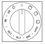
If you turn the control knob clockwise, it will automatically select a conventional oven function and you can regulate the temperature between 60 -250°C.
