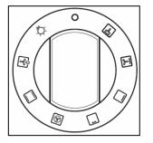
Use this control knob to select the oven function and turn on the oven light in the main oven.
