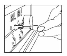
• Remove the knob from the tap and place a small bladed screwdriver down the centre of the tap shaft.
