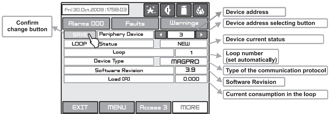
Fig. Screen 7 - LOOP (Loop controller) - Example for adding/ removing of new periphery device
