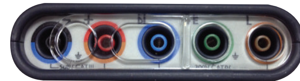
Fig.2 Interlock in position for RCD & Loop testing
