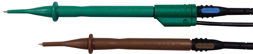
Fig 3. Prods in 2 wire testing configuration
