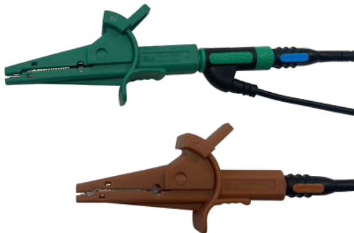
Fig 4. Crocodile clips in 2 wire testing configuration
