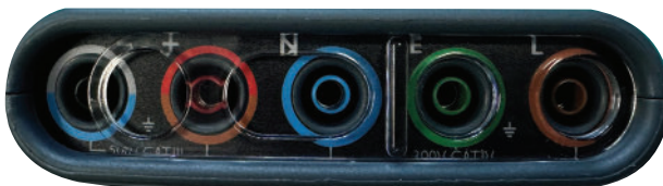
Fig.2 Interlock in position for RCD & Loop testing
