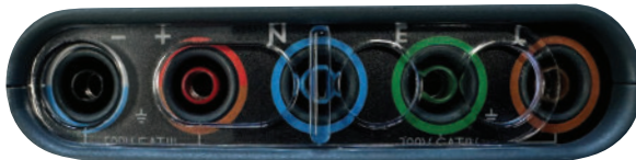
Fig.1 Interlock in position for Continuity and Insulation testing
