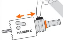
To remove the Hole Saw to use another diameter, just push the button and exchange the Hole Saw. Slide on another Hole Saw and you are ready to go.
