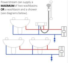
If connected to a mixer tap, it should be a **NON**-Thermostatic mixer tap; water mixes at the outlet pipe only.
