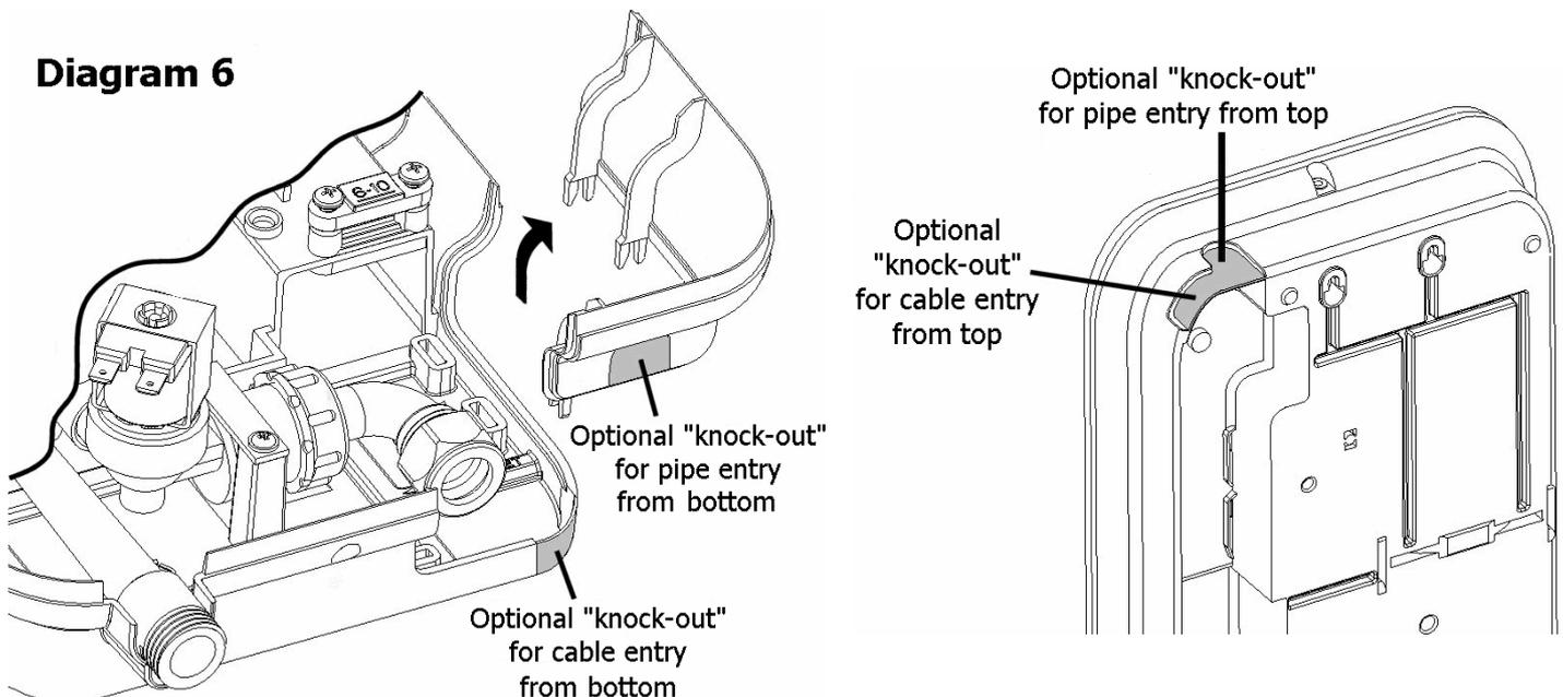
5. Decide the position of the electrical cable into the unit. If top or bottom entry is chosen (according to diagram 4), cut away the walls in the backplate as shown in diagram 6.
